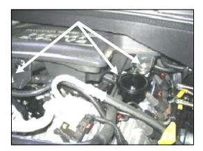
**6.** Remove the oil fill cap from the valve cover. Using a 10mm socket, loosen the two factory resonator bolts. Remove the resonator from the engine and then replace the oil fill cap.
