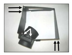
9. Assemble the Airaid Quick Fit Panels (#2, #3) using four  $6-32 \times 5/16$  'screws (#10),#6 flat washers (#11), and 6-32 keps nuts (#12). Next, install the air filter adapter (#4) using two  $\frac{1}{4}-20 \times \frac{1}{2}$  'button head screws (#13) and  $\frac{1}{4}$ " flat washers (#14).
