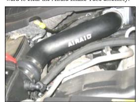
**15.** Install the Airaid Intake Tube assembly onto the engine with the hump hose end towards the air filter adapter. Adjust the assembly for fit and then tighten the four hose clamps.
