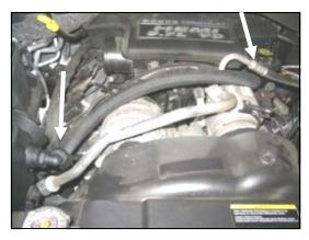
**12.** Remove the factory breather hose. Connect one end of the <sup>3</sup>/<sub>4</sub>" x 25" hose (#5) to the nylon fitting and the other to the oil fill nipple as shown. Secure each end using one #24 Speed Clamp (#16). Adjust the nylon fitting downward to clear the Airaid Intake Tube assembly.
