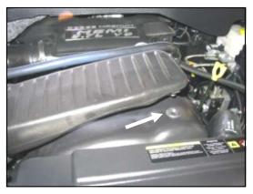
**2.** Unsnap the factory intake tube baffle from the fan shroud and then remove the factory intake tube assembly from the vehicle.
