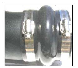
**14.** Install the hump hose (#7) and coupler (#8) onto the Airaid Intake Tube using four #60 hose clamps (#18). The coupler is positioned on the throttle body end and the hump hose is positioned on the air filter adapter end of the tube.
