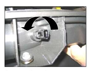
**7.** Remove the factory air temperature sensor from the resonator by turning it counter clockwise and pulling it straight out (save for reuse).
