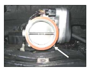
**8.** Remove the factory orange seal from the throttle body.
