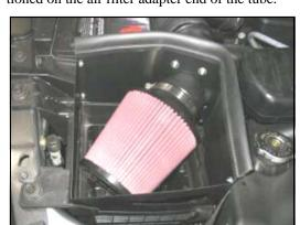
**17.** Install the Airaid Premium Filter (#1) onto the end of the air filter adapter. Install the weather strip (#9) onto the top of the Airaid Quick Fit Panels. (*Note: start from one end and work your way around to insure proper alignment of the weather strip.*)
