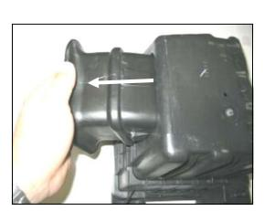
**4.** Using a flat blade screwdriver, carefully unsnap the air box base inlet from the air box base and remove it. Reinstall the factory air box base into the engine compartment without the inlet.
