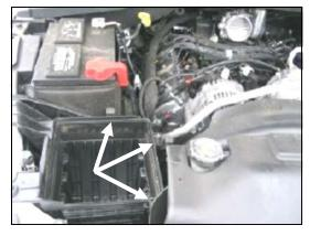
**3.** Unlatch the clips that secure the air box lid to the air box base, and remove the air box lid from the vehicle. Using a 13mm socket, remove the air box base from the engine compartment.
