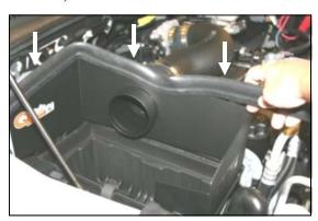
**14.** Install the weather strip (#6) onto the top of the Quick Fit Panel as shown. (*Hint: Start at one end and work towards the other.*)
