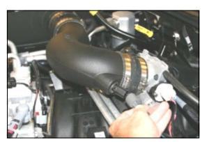
**13.** Reconnect the **AIT** sensor wiring harness to the sensor.
