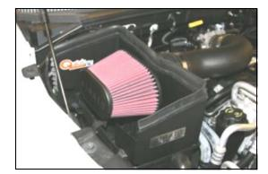
**15.** Install the Airaid Premium Filter (#1) onto the Quick Fit Panel as shown, and tighten the clamp.
