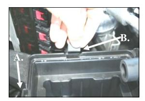
**5.** 2007 Models only: A.) Using a flat blade screwdriver, gently pry and remove one factory clip from the passenger side rear of the airbox base. (see arrow above)
