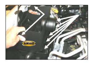
**6.** Slip the five tabs of the Quick fit panel (#2) through the slots on the airbox base. Adjust the panel for fit, then re-latch two of the factory clips onto the panel. Apply the Airaid Foil Decal onto the Panel as shown.
