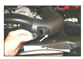
**8.** Install the grommet (#11) into the Airaid Intake Tube (#3).
