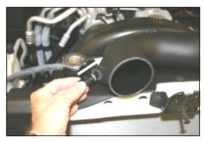
**10.** Carefully install the **AIT** sensor into the grommet in the Airaid Intake Tube. Make sure it goes all the way in.
