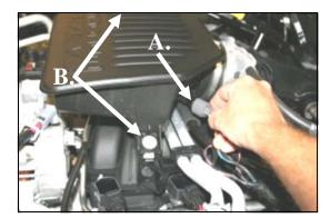
**4.** A.) Disconnect the <u>Air Intake Temperature</u> (AIT) sensor wiring harness.
