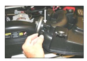
**9.** Carefully twist and remove the **AIT** sensor from the factory resonator.
