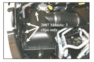
**1.** <u>Disconnect the negative battery cable.</u> Unlatch the four clips (three on 2007 models) on the factory airbox.
