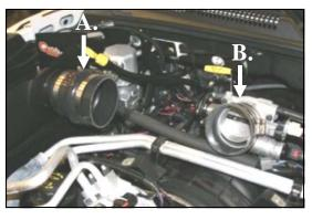
**11.** A.) Install the urethane hump hose (#5) and two #60 hose clamps (#9) onto the Quick fit Panel.
