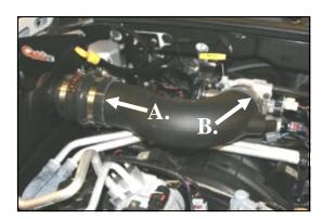
**12.** A.) Slide the Airaid Intake Tube into the hump hose first.
