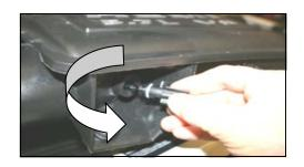
**6.** Gently twist the air temperature sensor counterclockwise and remove it from the
