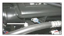
**3.** Squeeze the tab on the connector, and disconnect the intake temperature sensor.
