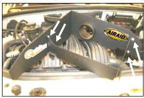
**7.** Assemble the Quick Fit Panels (#2 & #3) as shown, using the four provided screws (#8), washers (#9), and nuts (#10). Apply the Airaid Foil Decal onto the Panel as shown.
