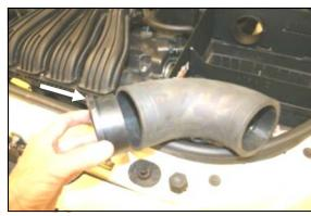
**9.** Install the reducer bushing (#5) into large end of the rubber elbow (#4).
