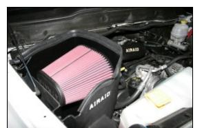
**16.** Install the Airaid Premium Filter (#1) onto the Airaid filter adapter, and tighten the hose clamp. Install the weather strip (#6) onto the top of the **CAD**, starting at the fender, and working your way towards the radiator.
