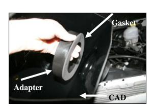
**6.** Install the filter gasket (#21) and filter adapter (#5) onto the Airaid Cool Air Dam (#3) as shown using three 1/4" x 5/8" bolts (#7), and 1/4" flat washers (#8). Refer to the line drawing above for reference.
