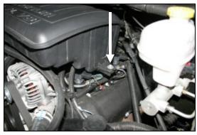
**4.** Using a 10mm socket, remove the two bolts that secure the intake resonator to the engine, one on the drivers side, and one on the passengers side of the resonator. Grab the resonator with both hands at the front and push back and up to release it from the locator grommet on the bottom. Remove the resonator from the vehicle.
