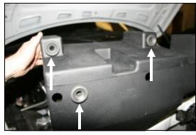
**8.** Install the factory grommets removed in step #3 into the bottom of the CAD at the locations shown here.
