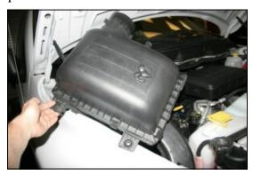
**2.** Slide the flexible intake tube off of the airbox lid and then lift the complete airbox straight up and out of the vehicle.
