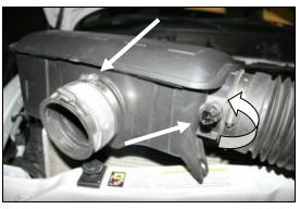
**5.** Loosen the factory hose clamp on the coupler and remove the coupler assembly from the resonator. **2003-07 Models** Next gently push in on the temperature sensor and rotate it to the left and remove it from the resonator. These parts will be reinstalled on the Airaid intake tube in step #12.
