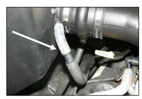
**14. 2004-07 Models;** Reconnect the factory breather hose to the 1/2" barbed fitting on the **CAD** using the 1/2" rubber elbow (#13), and 1/2"x 3/4" barbed fitting as shown.
