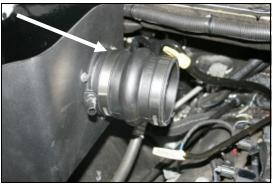
**11.** Install the hump hose onto the **CAD** using two #60 hose clamps (#9). Tighten the hose clamp on the **CAD**.
