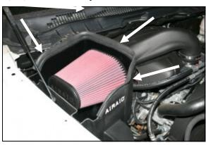
17. Install the Airaid Premium Filter (#1) onto the filter adapter and tighten the clamp. Next install the weather strip (#8) on the top of the CAB as shown. (Hint: Start at one end of the CAB and work your way towards the other end.)
