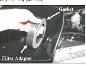
**7.** Install the adapter gasket (#19) and filter adapter (#6) into the **CAB** using three 1/4-20 x 5/8" bolts (#9) and flat washers (#10) as shown. *Refer to the line drawing above for reference*.
