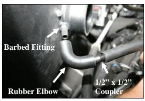
**12.** Install the supplied 1/2" x 1/2" plastic coupler (#16) into the 1/2" hose from step #11. Next connect the 1/2" rubber elbow (#15) between the 1/2" connector and the barbed fitting on the filter adapter.
