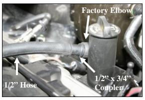
11. Remove the factory hard plastic breather tube from the rubber elbow behind the oil filler neck and then install the supplied 1/2" x 3/4" plastic reducing coupler (#18), into the factory rubber elbow as shown. Next, connect the supplied 1/2" x 22" hose (#7) to the coupler.
