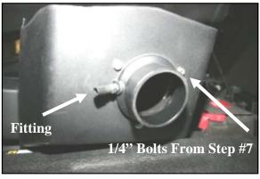
**8.** Install the 1/4" NPT x 1/2" barbed fitting (#17) into the filter adapter as shown.
