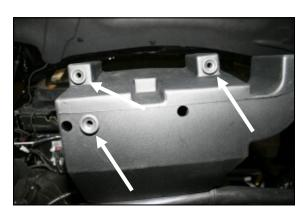
**6.** Install the three grommets removed in step #5 into the bottom of the Airaid Cool Air Box (CAB) (#3) at the locations shown here.
