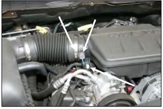
**5.** Reinstall the resonator and tighten the bolt that secures it to the intake manifold. Reinstall the intake tube, tighten the hose clamp, and reconnect the intake temperature sensor. **Re-connect the negative battery cable!**
