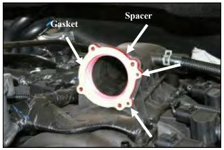
**3.** Install the Airaid Spacer into the intake manifold as shown. Make sure the spacer is seated correctly over the two alignment pins on the intake manifold. \*Note: Airaid spacer must be installed with bore protruding into intake manifold away from throttle body. Incorrect installation will hinder performance.
