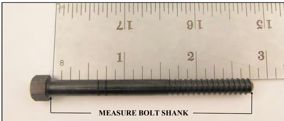
**3. Measure your OEM hardware to determine which Airaid bolts you will need. Measure the shank only. Use the chart below to select the proper bolts.**
