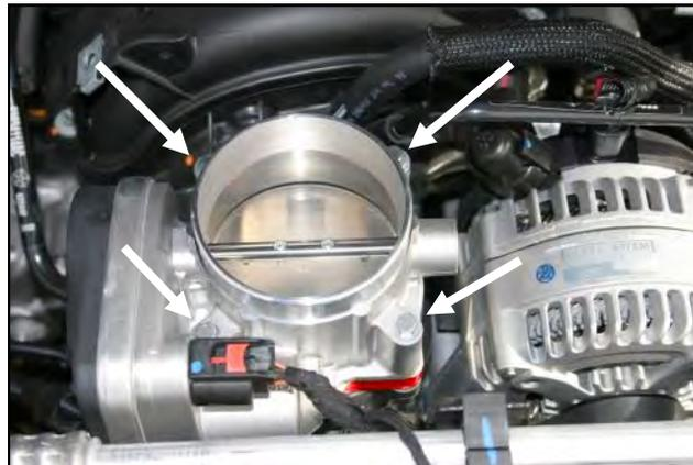
**5. Reinstall the throttle body on top of the Airaid Spacer using the four bolts and the washers that were selected in step 3. Tighten the bolts evenly, in an X pattern, to the vehicle manufacturers specifications.**
