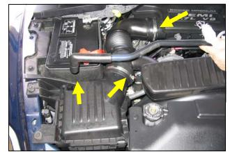
**1. Disconnect The Negative Battery Terminal!** Remove valve cover breather hose from air box lid. Loosen hose clamps on both sides of factory intake tube.
