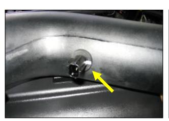
**7.** Install the supplied grommet and factory air temperature sensor into the Airaid MIT.
