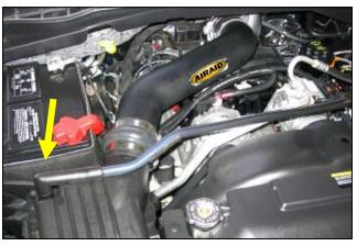
**11.** Adjust hose assembly for final position and tighten all four hose clamps. Reconnect valve cover breather hose to air box lid and replace oil fill cap.
