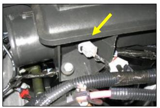
**3.** Carefully disconnect electrical connector from air temperature sensor in factory housing.
