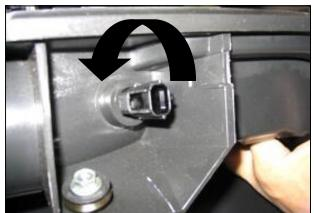
**5.** Remove air temperature sensor from housing by turning counter clockwise and pull.
