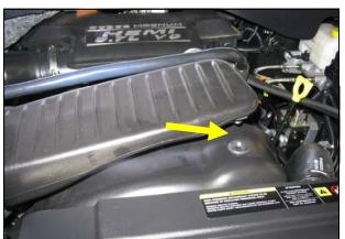
**2.** Unsnap factory air box tube baffle from fan shroud and remove air tube assembly from vehicle.
