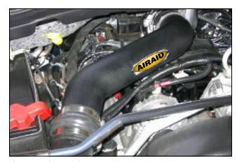
**9.** Check for any foreign objects or debris it the intake path & install Airaid MIT assembly on engine. (*Note: Leave hose clamps loose until final assembly*) Apply the Airaid Bubble Decal onto the Intake Tube as shown.
