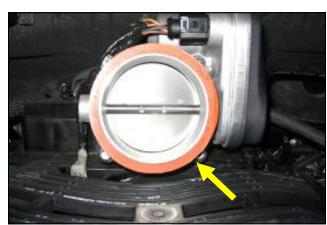
6. Remove factory orange seal from throttle body.
