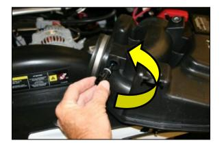
**5.** With the resonator turned over, carefully remove the air temp sensor by pushing in, and
