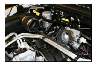
**6.** Install the urethane hump hose on the factory airbox with the two #60 hose clamps.
