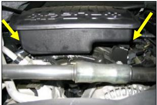
**5.** Loosen the two 10mm bolts mounting the factory air box to the intake manifold and remove from vehicle.
