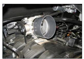
7. Install the reducer hose and a #52 hose clamp onto the throttle body. Install a #56 hose clamp onto the other side of the reducer.
