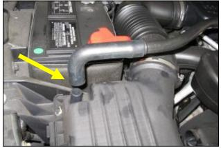
**1.Disconnect The Negative Battery Terminal!** Remove the breather hose from the factory air box lid.
