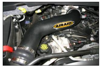
9. Install Airaid intake tube assembly by connecting the Airaid hump hose onto the factory air box lid and the other end onto the Airaid reducer hose. Tighten all hose clamps. Apply the Airaid Bubble Decal onto the Intake Tube as shown.
