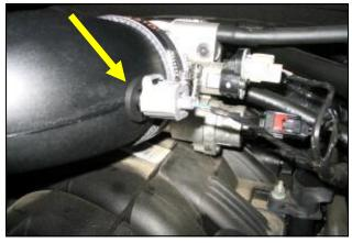
10. Install the supplied rubber grommet and factory air temperature sensor into the Airaid intake tube. Then, reconnect the factory electrical connector onto the sensor. Lastly, reconnect the factory breather hose to the air box lid.
