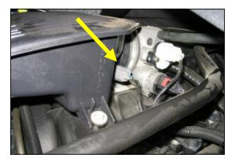
**4.** Disconnect the factory electrical connector from the factory air temperature sensor.
