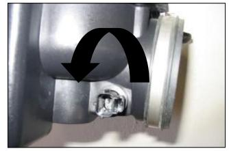
**6.** Turn the air temperature sensor ½ turn and remove from the air box. Retain sensor for later use.
