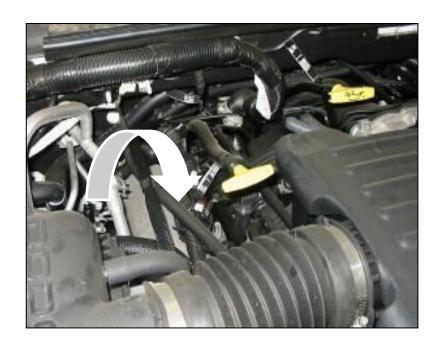
If your vehicle is equipped with a dipstick tube that interferes with the location of the Airaid Intake System, an adjustment to the dipstick tube must be made. Firmly grasp the dipstick tube about 6 inches below the top with vour left hand and carefully bend the tube towards the engine with your right hand. This will allow for clearance of the Airaid Intake System. Please refer to the image.
