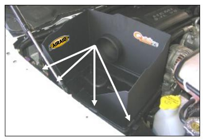
**3.** Position the Airaid Cool Air Dam (CAD) (#2) onto the factory airbox base. Relatch the factory clips onto the CAD. Apply the Airaid Foil Decal onto the Panel as shown.
