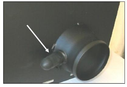
**5.** <u>2002-2003 Models Only</u>: Slip the black rubber cap (#6) over the nipple on the CAD and secure it using one #19 speed clamp (#5).
