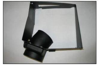
**4.** Using the supplied #6 screws, nuts and washers, assemble the two panels as shown above. Next, install the supplied air filter adapter using the supplied ½-20 bolts and washers.
