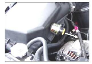
2. Remove the factory filter minder and rubber grommet (save for reuse).
