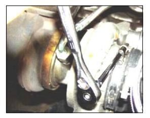
3. Using a 7mm socket, loosen the hose clamp where the factory intake tube connects to the turbo housing.
