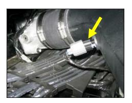
**16.** Re-connect air temperature sensor connector.
