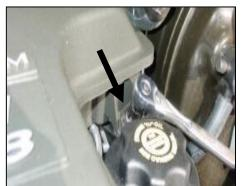
**2.** Loosen the two 10mm bolts securing the factory resonator to the intake manifold.
