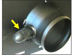
**10. 2003 Models Only:** Slip the black rubber cap over the nipple on the Cool Air Dam and secure using the #19 black speed clamp provided.
