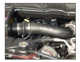
15. Slide the Airaid tube with hump hose into the Airaid Cool Air Dam first, and then slide the other end into the throttle body coupler. (Note: The Airaid tube should be flush against throttle body with a gap between the tube and Cool Air Dam assembly for engine movement.) After inspection, adjust the Airaid tube, coupler, and hump hose and tighten all hose clamps
