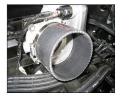
**14.** Slide the urethane coupler onto the throttle body and secure using a #60 hose clamp provided & install the 2nd #60 hose clamp on the other end of the coupler, leave loose for final assembly.
