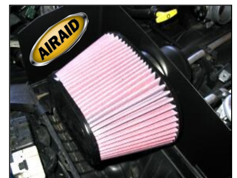
8. Mount the Airaid Premium filter inside the Cool Air Dam and secure with hose clamp provided. Apply the Airaid Foil Decal onto the Panel as shown.
