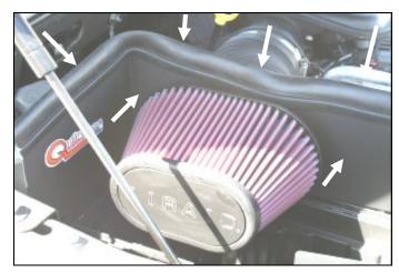
**8.** Install the Airaid Premium Filter (#1) onto the Quick Fit Panel as shown, and tighten the clamp. Install the weather strip (#3) onto the top of the Quick Fit Panel as shown. (*Hint: Start at one end and work towards the other.*)
