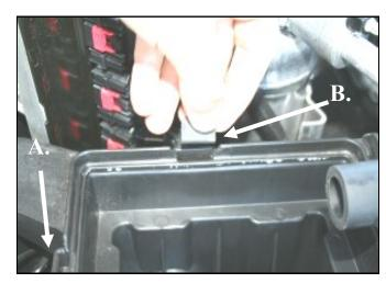
**4.** 2007 and newer models only: A.) Using a flat blade screwdriver, gently pry and remove one factory clip from the passenger side rear of the airbox base. (see arrow above) B.) Re-install the clip onto the rear of the factory airbox base (see arrow above).
