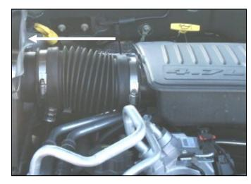
**6.** Slide the factory intake tube onto the Quick Fit Panel and tighten the hose clamp.
