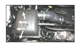
**2.** Unlatch 4 clips on the factory airbox lid and remove the lid and intake hose assembly. Re-
