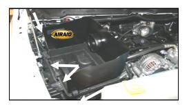
**8.** Install the Quick Fit Panel (#2) onto the factory airbox base by sliding the tabs on the base thru the Quick Fit Panel and then adjust the sides to fit. Re-latch the 4 clips to hold the Quick Fit Panel securely in place. Apply the Airaid Foil Decal onto the Panel as shown.
