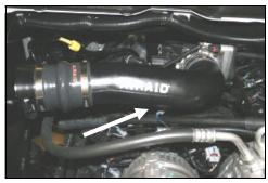
13. (Note: Because factory production tolerances vary, it may be necessary to remove the tape on the wiring loom and pull out 1 1/2" of wire to the temp sensor, and then re-install the tape. Re-connect the wiring harness to the temperature sensor.
