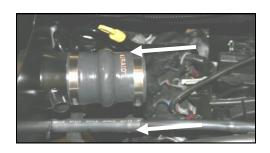
**9.** Install the urethane hump hose (#4) onto the tube on the Quick Fit Panel using two
