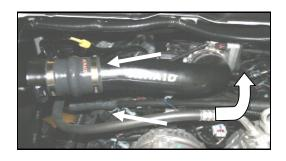
**11.** Install the Modular Intake Tube (#3) into the hump hose first and then into the reducing coupler. Adjust for fit, and then tighten all 4 hose clamps.
