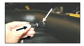
7. Install the supplied grommet (#12) into the Modular Intake Tube (#3). Next, carefully slide the factory temperature sensor into the grommet until it touches the tab on the temperature
