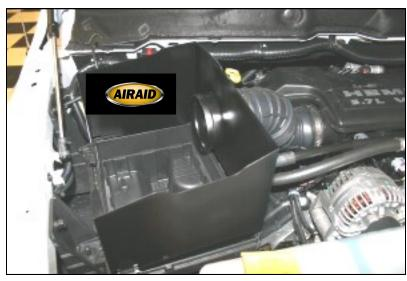
**4.** Install the **Quick Fit Panel** (#2) by slipping it into the factory intake tube, and then sliding it over the tabs on the factory airbox base. Adjust it for fit on top of the airbox base, and re-latch the 4 clips to hold the **Quick Fit Panel** securely in place. Apply the Airaid Foil Decal onto the Panel as shown.
