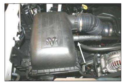
1. <u>Disconnect the negative battery cable!</u> Disconnect the factory breather hose from the air cleaner lid.
