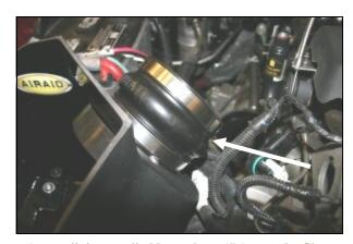
**10.** Install the supplied hump hose (#5) onto the filter adapter using two #72 hose clamps (#19). Leave the clamps loose for now. Apply the Airaid Bubble Decal inside the Airbox as shown.
