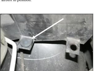
7. Install the supplied well nut (#16) into the factory airbox mounting hole closest to the fender as shown.
