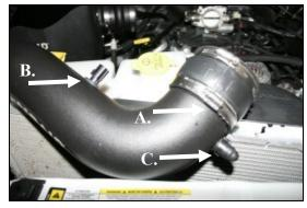
12. A.) Reinstall the factory coupler and hose clamps on to the Airaid intake tube (#2). Tighten the hose clamp on the tube. 2003-07 Models;
