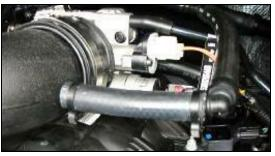
**15. 2002-03 Models;** Install one end of the provided 90° barbed fitting (#20) into the factory breather hose and then connect the supplied 1/2" breather hose (#19) to the other end. Connect the hose to the nipple on the Airaid intake tube. Secure all three connections with the provided #16 Speed Clamps (#15).
