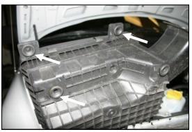
**3.** Turn the factory air box over and remove **3** of the 4 grommets. They will be reinstalled in the Airaid Cool Air Dam in step #8.
