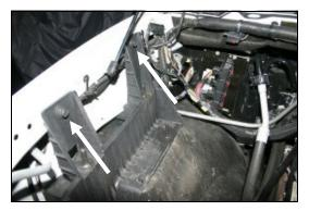
**9.** Remove the two bolts that secure the airbox mounting bracket to the inner fender. They will be reinstalled in step #10.
