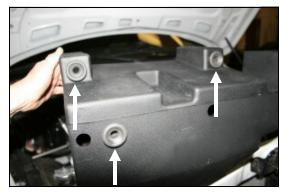
**8.** Install the factory grommets removed in step #3 into the bottom of the CAD at the locations shown here.
