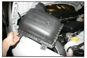
**2.** Slide the flexible intake tube off of the airbox lid and then lift the complete airbox straight up and out of the vehicle.
