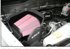
**16.** Install the Airaid Premium Filter (#1) onto the Airaid filter adapter, and tighten the hose clamp. Install the weather strip (#7) onto the top of the **CAB**, starting at the fender, and working your way towards the radiator.
