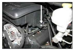
**4.** Using a 10mm socket, remove the two bolts (one bolt on 2008 and newer models) that secure the intake resonator to the engine, one on the drivers side, and one on the passenger side of the resonator. Grab the resonator with both hands at the front and push back and up to release it from the locator grommet on the bottom. Remove the resonator from the vehicle.
