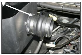
11. Install the hump hose (#4) onto the CAB using two #60 hose clamps (#11). Tighten the hose clamp on the CAB.
