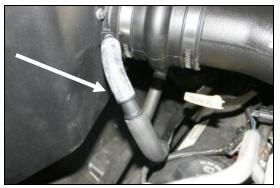
**14. 2004-12 Models:** Reconnect the factory breather hose to the 1/2" barbed fitting on the **CAB** using the 1/2" rubber elbow (#15), and 1/2"x 3/4" barbed fitting (#20) as shown.
