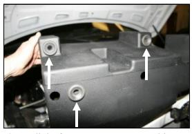
**8.** Install the factory grommets removed in step #3 into the bottom of the **CAB** at the locations shown here.
