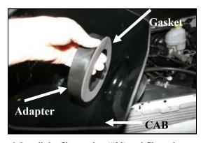
**6.** Install the filter gasket (#23) and filter adapter (#6) onto the Airaid Cool Air Box, or CAB (#3) as shown using three 1/4" x 5/8" bolts (#8), and 1/4" flat washers (#9). Refer to the line drawing above for reference.
