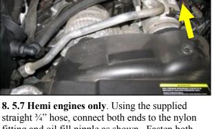
straight <sup>3</sup>/<sub>4</sub>" hose, connect both ends to the nylon fitting and oil fill nipple as shown. Fasten both ends using the supplied nylon speed clamps. Adjust the nylon fitting downward to clear the factory intake tube assembly.
