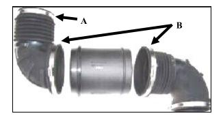
5. A.) Loosen the hose clamp that secures the factory airbox lid to the intake tube assembly, and remove the assembly from the lid.
