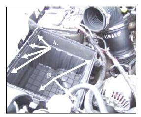
**12.** A.) Install the **CAD** by inserting the four tabs into the side of the factory airbox.
