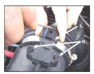
1. Disconnect the negative battery cable. A.) Disconnect the Intake Air Temperature (IAT) sensor wiring harness by pushing down on the tab, and sliding the connector back.
