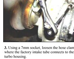
**3.** Using a 7mm socket, loosen the hose clamp where the factory intake tube connects to the
