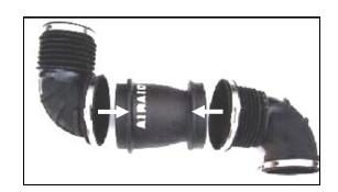
6. Replace the factory silencer tube with the Airaid Intake tube (#4). Complete the Airaid Intake tube assembly by aligning the notches in the tubes, and tightening the factory hose clamps.
