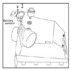
**11.** Install the factory **IAT** sensor into the air filter adapter using two 8-32 button head screws (#12), and #8 flat washers (#13). Install the factory rubber grommet and filter minder into the air filter adapter.
