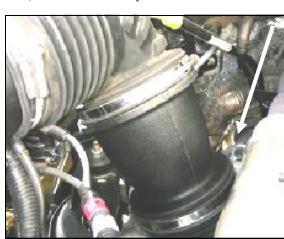
**8.** Install the Airaid Intake Tube assembly onto the turbocharger inlet. Tighten the factory hose clamp.
