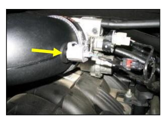
**15.** Install the supplied rubber grommet and factory air temperature sensor into the Airaid intake tube. Next, reconnect the factory electrical connector onto the sensor.
