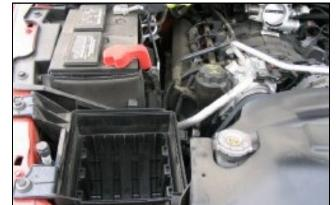
**3.** Unlatch the metal clips and remove the lid from air box base. Using a 13mm socket, remove the air box base from the engine compartment.
