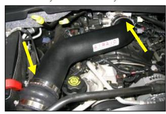
**14.** Install the Airaid intake tube assembly by connecting the Airaid hump hose onto the air filter adapter, and the other end into the Airaid reducing coupler. Tighten all hose clamps.
