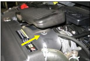
**2.** Unsnap the factory silencer box from the fan shroud and remove the factory tube assembly from the vehicle.
