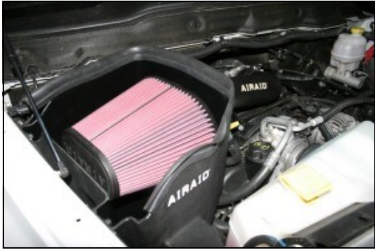
16. Install the Airaid Premium Filter (#1) onto the Airaid filter adapter, and tighten the hose clamp. Install the weather strip (#6) onto the top of the CAD, starting at the fender, and working your way towards the radiator.
