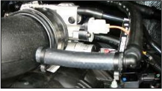
15. 2002-03 Models; Install one end of the provided 90° barbed fitting (#20) into the factory breather hose and then connect the supplied 1/2" breather hose (#19) to the other end. Connect the hose to the nipple on the Airaid intake tube. Secure all three connections with the provided #16 Speed Clamps (#15).
