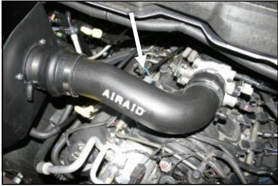
13. Slide the Airaid intake tube into the hump hose first, and then onto the throttle body. Adjust for fit, and then tighten the two remaining hose clamps. 2003-07 Models; Reconnect the temperature sensor wiring harness to the sensor in the tube.
