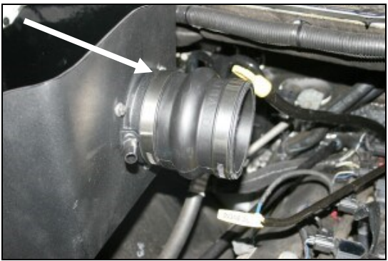
11. Install the hump hose onto the CAD using two #60 hose clamps (#9). Tighten the hose clamp on the CAD.
