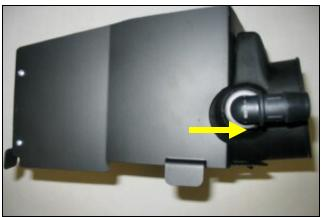
**9.** Install the supplied nylon fitting into the air filter adapter as shown.
