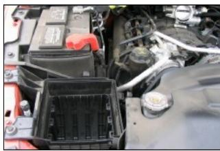
**3.** Unlatch the metal clips and remove the lid from air box base. Using a 13mm socket, remove the air box base from the engine compartment.
