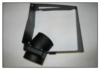
**8.** Using the supplied #6 screws, nuts and washers, assemble the two panels as shown above. Next, install the supplied air filter adapter using the supplied ½-20 bolts and washers.
