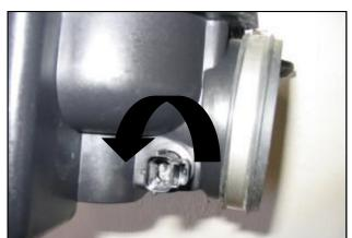
7. Turn the air temperature sensor ½ turn and remove from the air box. Retain sensor for later use.
