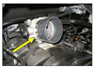
**12.** Install the supplied reducing coupler and #52 hose clamp onto the throttle body. Install the #56 hose clamp on the opposite end.
