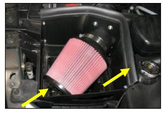
16. Install the Airaid Premium Filter on the end of the air filter adapter. Install the supplied weather strip on the Quick Fit panel. (Note: start from one end and work your way around to insure proper alignment of weather strip.)
