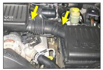
**1.** Disconnect the negative battery cable, and then loosen both of the hose clamps to factory tube connecting factory air filter assembly to factory air box silencer.
