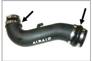
**8.** Slide the urethane hump hose and hose reducer onto the Modular Intake Tube. Use the two #60 hose clamps on the hump hose and a #56 & #52 hose clamp on the big & small ends of the reducer.
