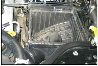
**2.** Remove the factory air filter box lid, accordion tube, and air filter. (Note: leave factory air filter base installed in vehicle)
