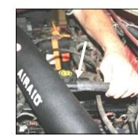
**21.** Re-connect the breather hose to the Airaid Intake Tube.
