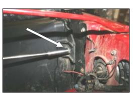
**9.** Remove one bolt from the passenger side radiator fan shroud and save it for step #15.
