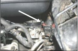
**3.** Loosen the clamp that holds the resonator to the throttle body.
