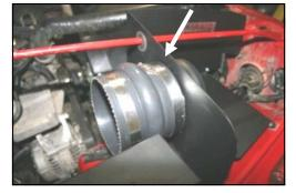
**16.** Install the hump hose (#5) onto the back side of the **CAD** tube using two #72 hose clamps (#17). Tighten <u>only</u> the hose clamp on the metal tube for now.
