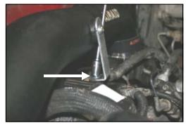
**20.** Install the 6mm bolt (#15), and 1/4" flat washer (#12), thru the L-bracket, and into the valve cover, adjust for fit, and then tighten all hose clamps, and bolts.
