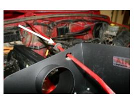
**12.** Slide the rubber grommet (#19) over the radiator support, followed by the assembled **CAD.** Use caution not to scratch the paint on the support rod.
