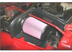
**22.** Install the Airaid Premium Filter (#1) onto the **CAD** tube and tighten the hose clamp. Next, install the weather strip onto the top of the CAD as shown, starting at the fender, working your way towards the radiator.
