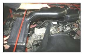
**2.** Unlatch the clips on the factory air cleaner lid, next remove the lid, and tube as an assembly.
