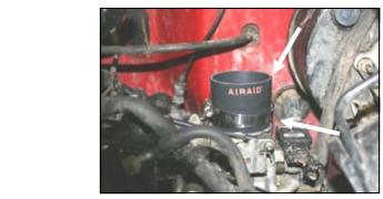
**17.** Install the reducer (#6) onto the throttle body using two #44 hose clamps (#16). Tighten only the hose clamp on the throttle body for now..
