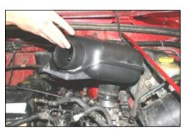
**6.** Remove the resonator from the vehicle.
