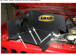
**11.** Assemble the two Cool Air Dam panels (#2) & (#3) using the four 6-32 screws (#8), #6 flat washers (#9), and nuts (#10). Apply the Airaid Foil Decal onto the Panel as shown.
