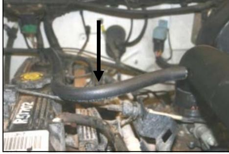
**17.** Replace the factory breather hose with the 1/2"x 14" breather hose (#8) between the valve cover and the intake tube using two #16 speed clamps (#21) as shown.
