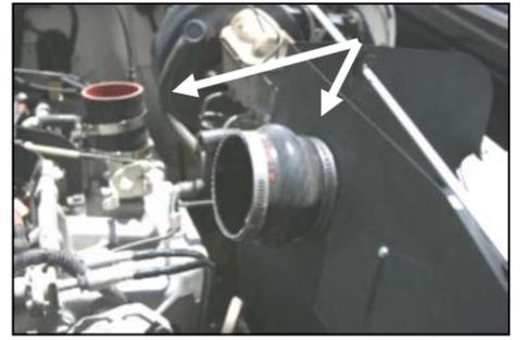
**15.** Install the urethane hump hose (#6) on the CAD with two #60 hose clamps (#18), and the coupler (#7) on the throttle body with two #44 hose clamps (#17). Leave the clamps loose for now.
