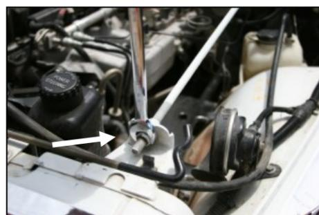
**8.** Using a 9/16" wrench, loosen the nut on the radiator support rod, and lift it up out of the slot.
