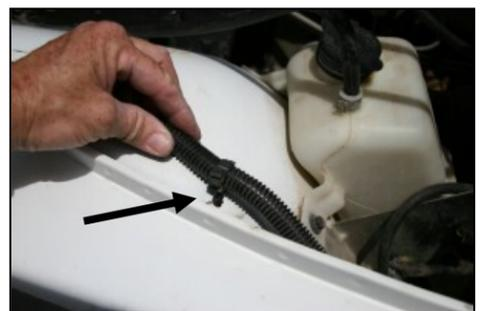
**6.** Carefully remove the wire loom clamp from the hole in the inner fender. Use caution not to damage the clamp, as it will be reused.
