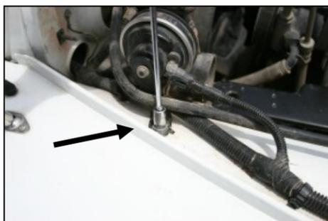
**5.** Using a 10mm socket, remove the horn bolt from the fender. (Save for later use.)
