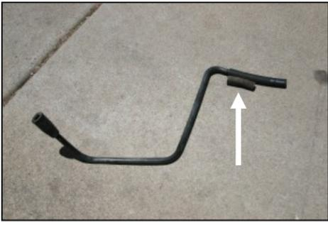
**13.** Remove the factory hose from step 2, and install the new 3/8"x4" hose (#23) on the end of the vacuum line as shown. Re-install the vacuum line. (Refer to step 2.)
