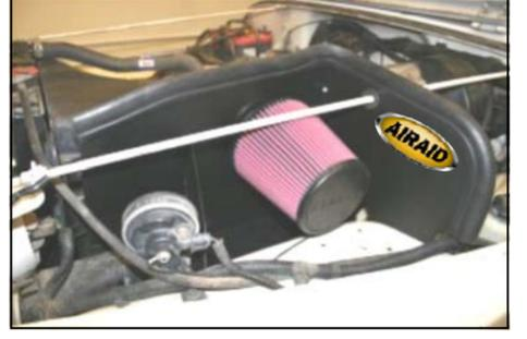
**18.** Install the Airaid Premium Filter (#1) and the weather strip (#9) onto the CAD, as shown. Apply the Airaid Foil Decal onto the Panel as shown.
