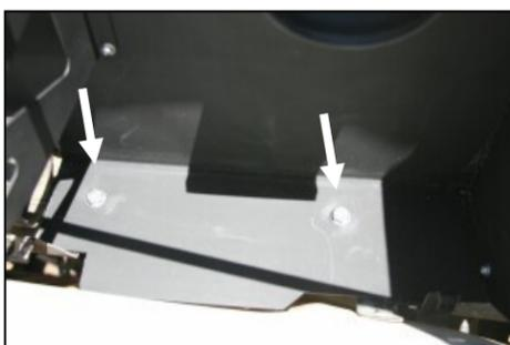
**10.** Install two 1/4 - 20 x 5/8" hex bolts (#13) and 1/4" flat washers (#14) thru the top of the CAD, and fender washers (#15) and lock-nuts (#16) on the bottom, where the factory grommets were removed.
