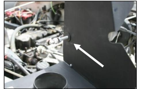
**9.** Carefully slide the CAD over the support rod, and then slide the supplied grommet over the rod, and into the hole in the CAD as shown. Rotate the CAD and place it into position on the factory airbox mount. Re-install the radiator support rod, and tighten the nut.
