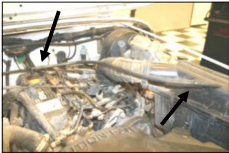
**1. Disconnect the negative battery cable.** Remove the factory valve cover breather hose from the airbox, and the valve cover.
