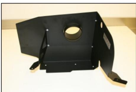
**7.** Assemble the Cool Air Dam (CAD) panels (#2, #3, & #4) as shown using the 5 provided screws (#10), washers (#11), and nuts (#12).
