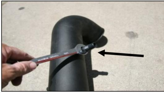
**14.** Install the 1/4" barbed fitting (#22) into the intake tube.
