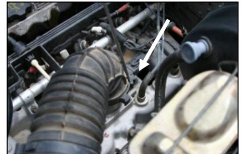
**3.** Pry open the plastic clamp that holds the factory intake tube to the throttle body. Unhook the 3 metal latches on the airbox that hold it to the mounting plate, and remove the intake assembly.
