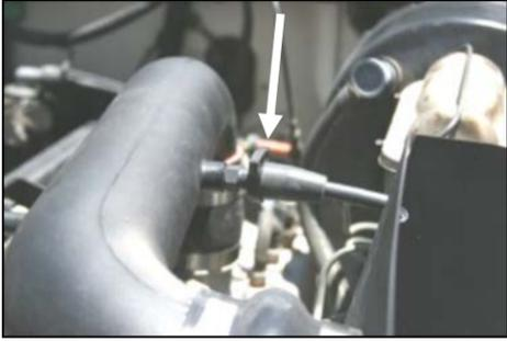
**16.** Slide intake tube into the hump hose first, and then into the coupler. Adjust for a good fit, and tighten the hose clamps. Slide the vacuum hose on the barbed fitting, and install one #16 speed clamp (#21) as shown.
