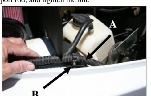
**12.** A) Using a 1/4-20 bolt (#13), 2 washers (#14), and locknut (#16), bolt the CAD to the fender. B) Install the wire loom clamp into the hole in the CAD, as shown.
