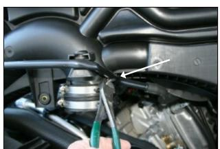
**8.** Carefully pull the resonator towards you and rotate the bottom up to gain access to the tie wrap holding the breather hose to the rubber coupler. Cut the tie wrap and discard.
