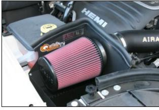
**19.** Install the Airaid Premium Filter on the Quick Fit assembly as shown, and tighten the hose clamp.
