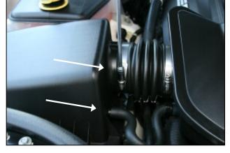
**1.Disconnect The Negative Battery Terminal!**Loosen the hose clamp on air cleaner box lid. Twist and remove breather hose from air cleaner box lid.
