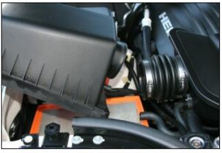
**3.** Remove the air cleaner box lid by sliding it forward, and then up, and out of the factory intake tube.
