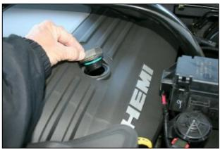
5. Remove, and set aside the oil filler cap. *Use caution not to drop anything into engine while cap is off.*
