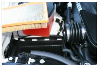
**4.** Remove factory air filter from air cleaner box.
