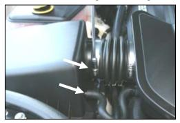
1. **Disconnect the negative battery cable.** Loosen the hose clamp on air cleaner box lid. Twist and remove the breather hose from the air cleaner box lid.
