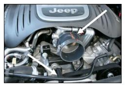
**15.** Install the reducer (#6) and two #56 hose clamps (#9) on the throttle body as shown. **Do not tighten** the clamps at this time. Secure the breather hose to the air conditioner line using the supplied zip tie (#15).
