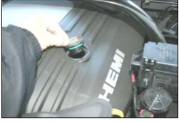
**5.** Remove, and set aside the oil filler cap. Use caution not to drop anything into the engine while the cap is off.
