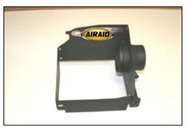
**11.** Assemble the two pieces of the Quick Fit panels as shown (#2&#3), using the four 6-32 screws (#12), washers (#13), and nuts (#14), that are provided in the kit. Apply the Airaid Foil Decal onto the Panel as shown.
