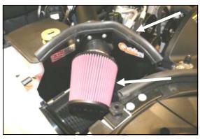
**17.** Install the Airaid Premium Filter (#1) onto the air filter adapter. Next, install the weather strip (#8) on the top of the Quick Fit panels as shown.
