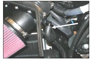
**18.** Reconnect the factory breather hose onto the 90° nylon fitting (#9).
