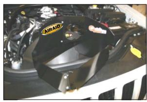
**9.** Assemble the Quick Fit panels as shown, using five 6-32 screws (#16), #6 washers (#17), and keps nuts (#18). Apply the Airaid Foil Decal onto the Panel as shown.
