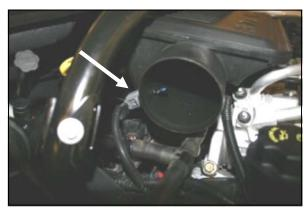
**6.** Disconnect the intake air temperature sensor wiring harness, by squeezing the tab on the side, and sliding the connector off.
