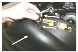
**15.** Install the rubber grommet (#12) into the Modular Intake Tube (#5). Next, slide the factory intake air temp sensor into the grommet in the tube. Make sure it is seated all of the way in.
