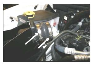
**13.** Install the provided hump hose (#7) onto the air filter adapter. Place a #60 hose clamp (#15) on each side of the hump hose. Tighten <u>only</u> the clamp on the air filter adapter. Leave the other clamp loose for now.
