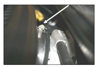
**7.** Using the 5/16" socket, ratchet and extension (or flat blade screw driver)- loosen hose clamp on the throttle body. This clamp is located close to the firewall, in the center of the engine compartment.
