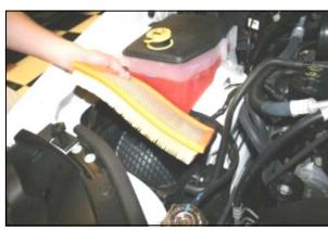
**5.** Remove the factory air filter.
