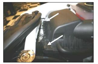
**2.** Unlatch the two clips on the factory air cleaner box lid.
