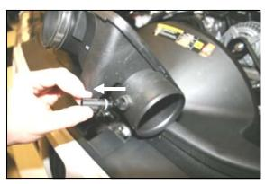
**14.** Remove the factory intake air temp sensor from the resonator box by carefully twisting the sensor body, and pulling it straight out of its mount. Place the sensor in a safe location, it will be re-used in step #15.
