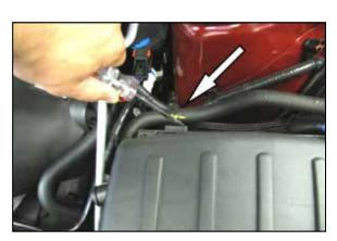
3. Using a standard head screwdriver, carefully pry and separate the hose anchor from the airbox lid. This anchor will be reused on the Airaid Intake System.
