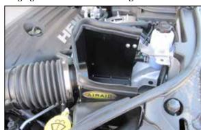
16. Install the Weather Strip (#4) to the top edge of the panels, and reattach the hood seal. Apply the Airaid Decal to the Panel Assembly.
