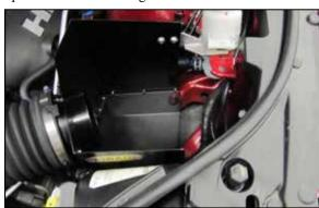
13. Install the Panel assembly into the engine compartment as shown. On vehicles equipped with a power steering reservoir, slide the Mounting bracket underneath the power steering reservoir and the airbox mounting post through the grommet in the Panel. Secure the assembly by reusing the bolt from step 12a. On vehicles that are equipped with electronic power steering, secure the assembly using the bolt from step 12b. Connect the factory intake tube to the Airaid Intake tube and tighten the clamp.
