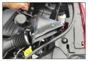
6. Unseat the lower half of the factory airbox from it's mounting grommets and remove the airbox and air inlet duct as an assembly.
