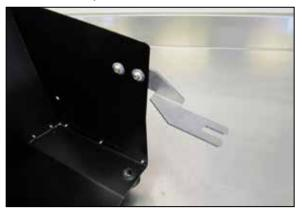
11. Install the Mounting Bracket (#6) onto the Panel assembly using the two 1/4-20 Button Head Bolts (#8), 1/4" Flat Washers (#9), and 1/4-20 Flange nuts (#10). NOTE: On vehicles that are equipped with "Electronic Power Steering" install bracket #13
