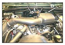
1. **Disconnect the negative battery cable!** A). Loosen the hose clamp that holds the factory intake resonator to the throttle body. B). Loosen the hose clamp that connects to the airbox. C). Remove two bolts on top of the valve cover. D). Disconnect the breather hose on the back of the resonator.
