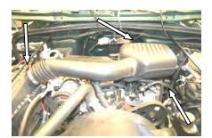
7. Re-connect the intake tube to the airbox, reconnect the breather hose, and tighten all hose clamps.
