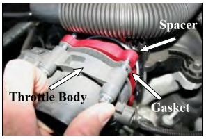
3. Install the AIRAID Spacer and the fiber gasket between the intake manifold, and the throttle body, as shown. Tighten all 4 throttle body bolts evenly, to the manufacturer's specifications. **Do Not Over Tighten The Bolts!** \*Note: AIRAID spacer must be installed with bore protruding into intake manifold away from throttle body. Incorrect installation will hinder performance. Reference picture below for spacer orientation.
