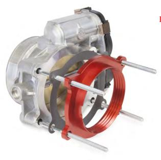
Example of proper spacer installation. Spacer must protrude into intake manifold and away from throttle body.
