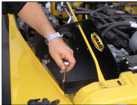
14. Using the supplied 1/4 x 20 nut, bolt and washers, mount the front of the Airaid Cool Air Dam to the inner fender.
