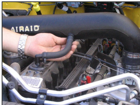
26. Connect the other end of the valve cover hose to the intake tube. Secure both ends of the hose using the supplied black speed clamps.
