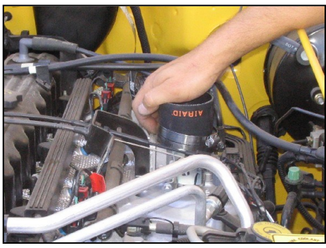
21. Install reducer coupler on throttle body with two #44 hose clamps. Leave hose clamps loose until final assembly.
