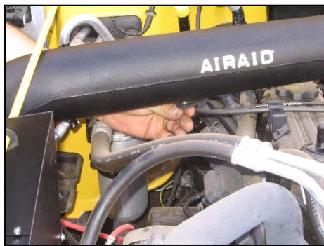
23. Mount the Airaid intake tube to the valve cover bracket using the supplied 1/4" bolt and washer as shown above.
