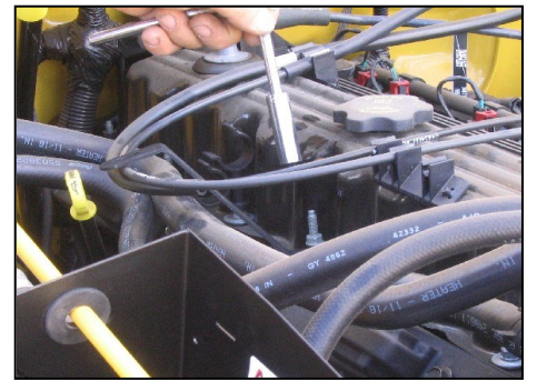
16. Remove one valve cover bolt on the passenger side nearest to the oil fill cap. Use this bolt to mount the supplied mounting bracket to the engine as shown above. Leave bolt loose until final assembly
