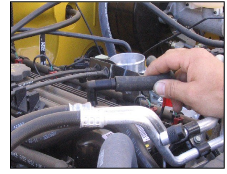
19. Install the supplied rubber hose on the factory plastic valve cover breather fitting.
