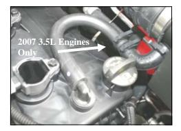
**8. For 2007 3.5L Engines**, (shown above), slide one end of the 1/2"x 1/2" connector (#10) into the rubber elbow. Slide the other end into the factory breather hose. Install one speed clamp (#9) over the factory breather hose and 1/2" connector as shown.
