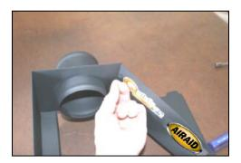
**5.** Assemble the Quick Fit panels (#2, #3) using four 6-32x 5/16" screws
