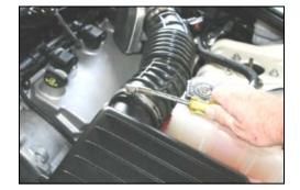
**2.** Loosen the hose clamp on the factory intake tube, located at the air box lid.
