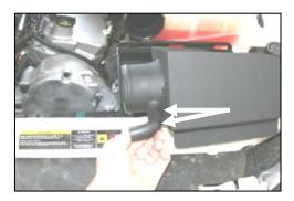
**6.** Slide the 1/2" rubber elbow (#8) onto the breather fitting on the side of the
