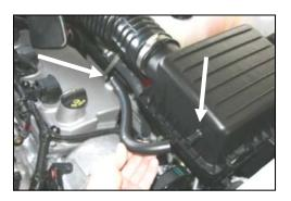
Disconnect the negative battery cable. Remove the breather hose from the factory air box lid and valve cover.
