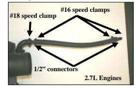
**9. 2.7L Engines:** Install the two 1/2" connectors (#12),into each end of the supplied breather hose (#4). Connect the breather hose to the rubber elbow on the Quick Fit Panel using one #18 speed clamp (#10), and one #16 speed clamp (#11). Install one #16 speed clamp on the opposite end of the hose as shown.
