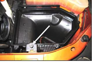
**2.** Remove the core support bolt securing the lower half of the airbox and remove it from the vehicle.
