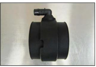
**13. For 6.4L V8 SRT-8 equipped vehicles:** Locate the V8 Airaid Intake Tube marked KIT-210-8T and insert the larger, 3/4" Grommet into the side. Complete the SRT-8 Tube assembly by inserting the 5/8" 90 Degree, Barbed Fitting into the Grommet as shown.
