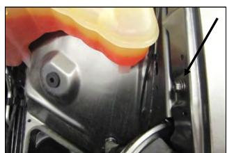
**8.** Remove and save the factory 6mm fender bolt. It will be reused in step **9**.
