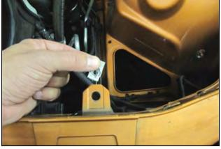
**3.** Carefully remove the speed clip from the core support tab and set it aside. It will not be reused.
