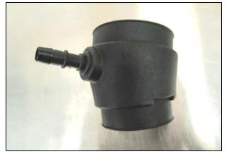
11. For 3.6L V6 Pentastar equipped vehicles: Locate the V6 Airaid Intake Tube marked KIT210-6T. On vehicles that the crank case vent is connected to the factory air box, insert the smaller 5/8" grommet into the tube and then complete the assembly with the 5/8" barbed fitting. On vehicles that have the crank case vent connected into the factory intake tube, install the provided plug (082007) into the Airaid intake tube.
