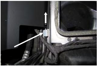
10. Snap the Line Holder onto the ABS line closest to the panel assembly and remove the adhesive backing. Gently push the Panel away from the line and slide the Line Holder behind the Panel. Relax the Panel, and allow the Adhesive pad to bond the Panel. This will isolate the Panel and prevent contact with the ABS line.
