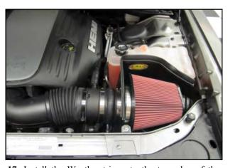
17. Install the Weatherstrip onto the top edge of the Panels with the contour rolling away from the Filter area. Complete the installation by attaching the Airaid Premium Filter to the Filter Adapter.
