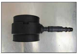
**12.** For **5.7L V8 HEMI equipped vehicles:** Locate the V8 Airaid Intake Tube marked KIT-210-8T and insert the larger, 3/4" Grommet and one of the larger, 3/4" Barbed fittings into the side. Complete the V8 Tube assembly by installing the 2 1/2", 3/4" Hose onto the Tube Fitting, and inserting the second 3/4" Barbed Fitting into it as shown.
