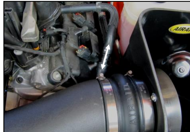
15. Connect the Barbed Fitting in the PCV hose to crank case breather line in the valve cover .
