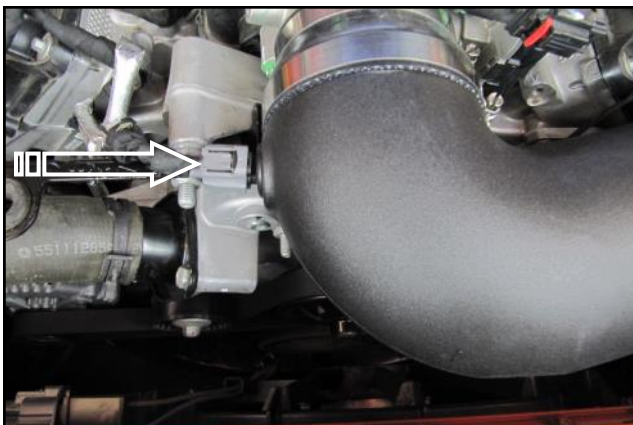
14. Reconnect the air temperature sensor.
