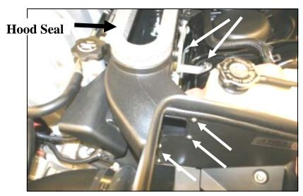
Install the hood scoop into the **CAD** using three 8-32 x 3/8" button head screws (#2), and three #8 flat washers (#3), leave loose. Install the L-bracket (#6) over the stud on the fender, and bolt it to the hood scoop using the 1/4-20 button head bolt (#4), and 1/4" flat washer (#5). Replace the factory nut on the stud, adjust for fit, and tighten all bolts, nuts, and screws. Apply the Foam Hood Seal as shown.
