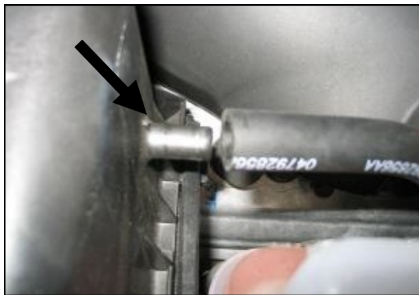
2. Disconnect the breather hose from the factory air box lid.
