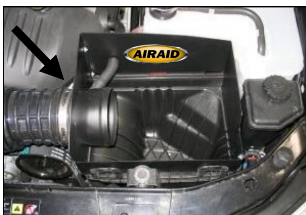
5. Install the Airaid CAD in place of the factory air box lid. Tighten factory hose clamp. Apply the Airaid Foil Decal onto the Panel as shown.
