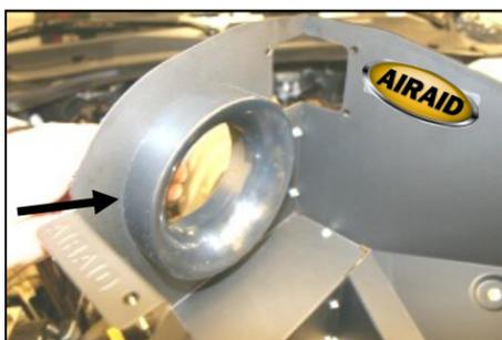
**8. Next install the filter adapter (#6) using three 1/4 - 20 button head bolts (#12), and 1/4" flat washers (#13).**
