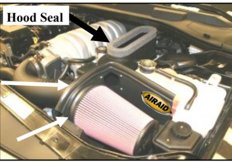
**17.** Install the Airaid Premium Filter (#1), onto the filter adapter inside of the CAD, and tighten the hose clamp. Next install the weather strip (#9) onto the top of the CAD. apply the hood seal onto the top side of the Hood Scoop.
