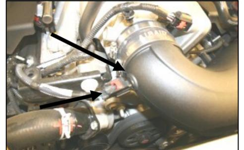
**15.** Install the grommet (#21) into the hole in the Airaid Intake Tube, and then gently push the temperature sensor (*removed in step #4*) thru the grommet until completely seated.
