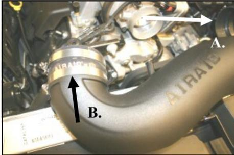
**13. A.** Install the urethane hump hose (#7) on the filter adapter using two #72 hose clamps (#20), (*Leave loose for now*). **B.** Install the reducing coupler (#8) large end on the Airaid Intake Tube (#4), using two #52 hose clamps (#19). Tighten *only* the hose clamp on the tube.
