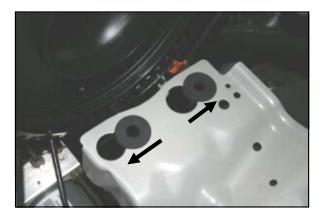
**9.** Slip two rubber grommets (#14) into the large holes in the factory airbox mounting plate, and then slide them sideways into the small holes as shown.
