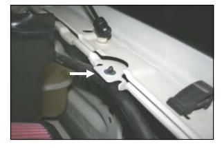
**15.** Slip the black plastic hose mount (#17) over the radiator overflow hose. Next, place one  $\frac{1}{4}$ " flat washer (#10) over the hole on the inner drivers side fender. Slide the hose mount prongs thru the fender and thru the washer.
