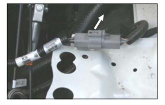
**8. 4.2L Engine Only**: Using a flat blade screwdriver, carefully pry the **MAF** sensor wiring harness connector from the holes in the airbox mounting plate (*do not disconnect it*). Move the harness towards the firewall to allow room for the **CAD** to mount.
