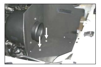
**12.** Insert two  $\frac{1}{4}-20 \ge \frac{7}{8}$ " bolts (#9) and  $\frac{1}{4}$ " flat washers (#10) through the holes in the CAD and thru the grommets. On the underside of the factory airbox mounting plate, align the long/narrow bracket (#16), two  $\frac{1}{4}$ " flat washers (#10), and two  $\frac{1}{4}-20$  nuts (#12) with the  $\frac{1}{4}-20 \ge \frac{7}{8}$ " bolts. Tighten the assembly securely.
