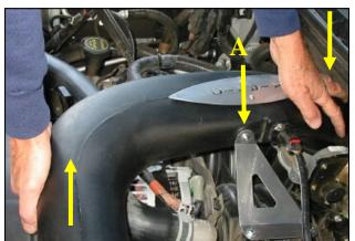
13. Install the Airaid intake tube over the throttle body, and into the hump hose. A.) Install the two ½-20 Allen bolts and washers thru the brackets and into the tube. Push down on the throttle body end, and lift up on the curve of the tube. Make sure the tube is seated all the way down on the throttle body! Tighten the Allen bolts, and then the tower bolts.
