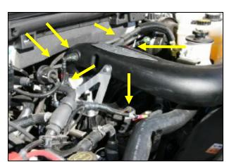
**15.** Reconnect the Mass Airflow Sensor and vacuum hose. Reconnect the breather line, and vacuum line in the clip. Reinstall the wire harness, and heater control valve on the tower bolts.
