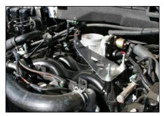
12. Install the two Airaid intake tube brackets on the top of the intake manifold, using the four aluminum spacers on top of the bracket and the four tower bolts. (Leave loose until final adjustments are made.)
