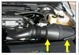
**2.** Grasp large oval section of intake tube and pull up and away from inner fender well, and remove entire intake tube. (*Note: Intake tube is held in with rubber grommets, no bolts.*)
