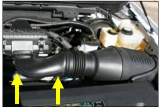
**1.Disconnect The Negative Battery Terminal!** Grasp intake tube and sharply lift up and away from airbox.
