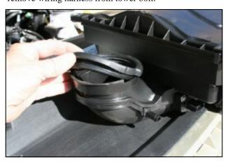
**7.** Remove the factory rubber seal from the airbox, and install it on the Airaid intake tube.
