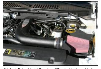
**16.** Install the Airaid Premium Filter inside the cold air dam. Apply the Airaid Foil Decal onto the Panel as shown.
