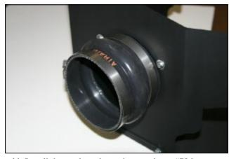
**11.** Install the urethane hump hose and two #72 hose clamps. (*Leave loose until final adjustments are made.*)
