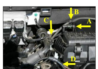
**4.** *A.*) Remove breather line by pushing up on green lever and pulling fitting away from airbox. *B.*) Remove vacuum line from clip. *C.*) Pull up on, and remove heater control valve from tower bolt. *D.*) Pull up on, and remove wiring harness from tower bolt.
