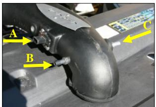
**8.** Remove the mass air sensor from the stock airbox using the #20 torx tool. *A.*) Using the supplied 8/32 screws install the mass air sensor in the Airaid intake tube. *B.*) Install the 3/8" plastic hose fitting. **Do not over tighten!** *C.*) Install the supplied grommet, and then the supplied aluminum fitting, rounded end first.
