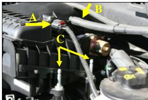
**5.** *A.*) Unhook the mass air flow sensor by pulling out the red plastic tab first, and then remove the plug. *B.*) Unhook the vacuum line. *C.*) Remove all four tower bolts and remove air box. (*Save tower bolts for reinstallation.*)
