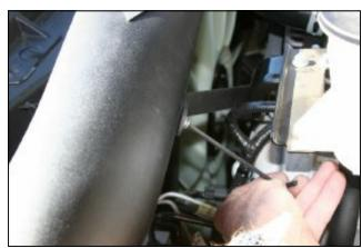
**14.** Install a ¼-20 Allen bolt and flat washer thru the bracket at the back of the tube, and tighten. Tighten the nut at the bottom of the bracket. Tighten the hose clamps on the hump hose.
