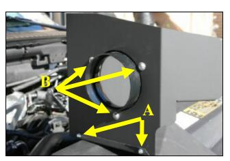
**9.** *A.*) Assemble the Cool Air Dam using the four 6-32 screws and locknuts. *B.*) Install the air filter adapter using three ½-20 Allen bolts and washers.
