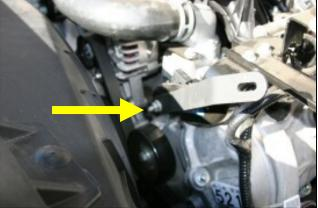
**3.** Remove 13mm nut on power steering reservoir bracket. Install Airaid intake tube support bracket, replace nut, and leave slightly loose. (*Nut will be tightened after final adjustments.*)
