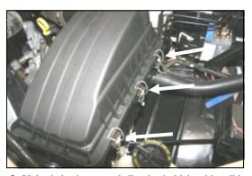
2. Unlatch the three metal clips that hold the airbox lid to the base.
