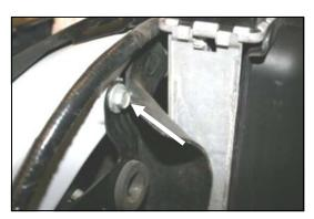
7. Using a 1/2" socket, ratchet, and extension, remove one bolt attaching the air cleaner base alignment bracket to the radiator support. The bolt will be reused in step #11.
