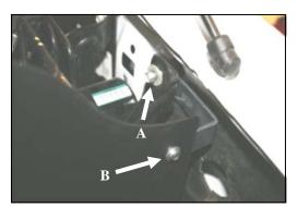
**12. A.**) Slide the L-bracket under the antilock braking system bracket, and re-install the bolt removed in step #8.
