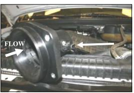
5. Install the factory mass air sensor into the Airaid MAF Adapter (#4), using the two supplied 8-32 button head screws (#9) and a 3/32" allen wrench. Note the direction of flow on the sensor, and mount as shown above. **DO NOT USE THE FACTORY SCREWS!!**
