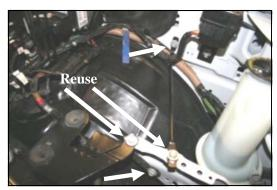
**6.** Using a 1/2" socket, ratchet and extension, remove the 2 bolts that hold the support rod, and 2 bolts that hold the air cleaner base support. Remove the support rod and base support and set them aside. The 2 bolts that hold the air cleaner base support will be reused in step #11.
