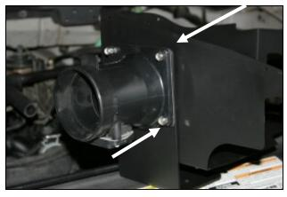
**7.** Assemble the MAF sensor housing, MAF gasket, MAF bracket and two panels as shown using the four bolts and nuts from step #5.
