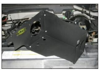
**6.** Assemble the two panels (#1) & (#2) as shown using four 6-32x3/8" Phillips head screws (#5), #6 flat washers (#6), and Kep nuts (#7). Apply the Airaid Foil Decal onto the Panel as shown.
