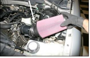
**3.** Loosen the hose clamp and remove the air filter from the vehicle.
