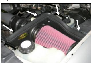
**11.** If you <u>Do</u> have a hood mat, install the Airaid Premium Filter onto the MAF bracket and tighten the filter. Next install the weatherstrip (#4) onto the top of the panel assembly as shown. *If your vehicle <u>Does Not</u> have a hood mat, proceed to step # 12.*
