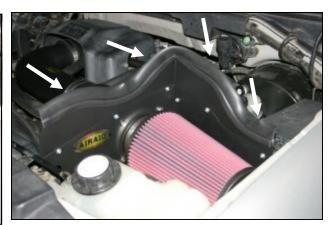
**12.** If your vehicle <u>Does Not</u> have a hood mat, install the panel extension (#4) as shown using five 6-32 Phillips head screws (#5), flat washers (#6), and kep nuts (#7). Next install the weatherstrip (#4) onto the top of the panel assembly as shown.
