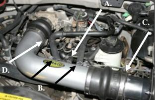
2.A). Disconnect the temperature sensor wiring harness from intake air temperature sensor.
