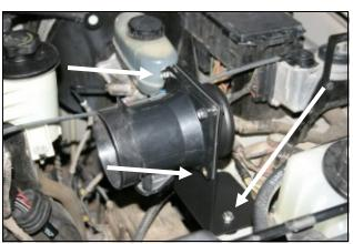
**5.** Remove the four bolts that secure the MAF sensor housing to the MAF bracket. Remove the MAF sensor housing and gasket and set them aside. These parts will be reused in step #7. Next remove the MAF bracket from the vehicle. The bracket and mounting hardware will be reused in step #9.
