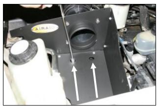
**9.** Reinstall the mounting hardware from step #5 securing the MAF bracket to the factory mounting bracket.
