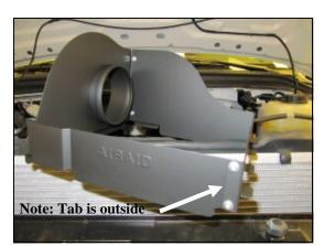
**4.** Assemble the two Quick Fit panels (#3 & #4) as shown using four 6-32 screws (#9) flat washers (#11) and kep nuts (#10).
