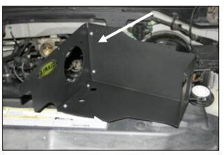
**6.** Assemble the MAF panel (#3), and bottom panel (#4) as shown using four 6-32 screws (#12), four flat washers (#13), and four Kep nuts (#14) as shown. Apply the Airaid Foil Decal onto the Panel as shown.
