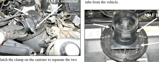
to the adapter. Separate the adapter plate from the MAF sensor housing and save the sensor and housing for reinstallation in step #7.
