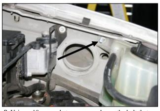
**8.** Using a 10mm socket, remove and save the bolt that secures the radiator overflow tank to the driver side inner fender well.
