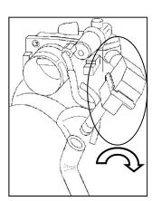
**15.** <u>4.6L engines</u>: The idle air bypass line goes directly to the throttle body. Rotate the resonator box 90 degrees to provide clearance for the 3/4 x 12" L-hose (#7). Install the 3/4"x12" L-hose (#10) onto the Airaid Intake tube and the resonator box and secure it using the two #22 speed clamps (#23)
