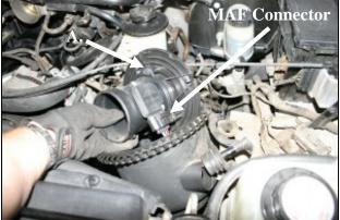
4.Unlatch the clamp on the canister to separate the two halves. Once separated, remove the factory air filter. A) Next, slide the large round plastic Mass Air Flow (MAF) sensor adapter plate from the canister. To do this, slide the wires thru the rubber grommet to gain access to the MAF sensor wiring connector. Now disconnect the MAF sensor wiring harness, and remove the MAF sensor housing and adapter plate. Remove the remaining half of the canister from the vehicle.
