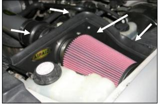
**16.** Reinstall the beauty cover using the 3 factory bolts. Install the Airaid Premium Filter (#1) as shown, and tighten the hose clamp.
