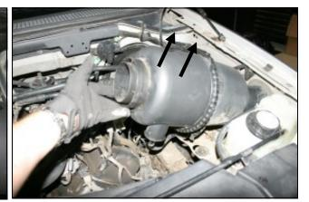
3. Lift straight up on the outlet side of the air filter canister to remove it from it's locating grommets. Next, pull it towards the engine to dislodge it from the inner fender
